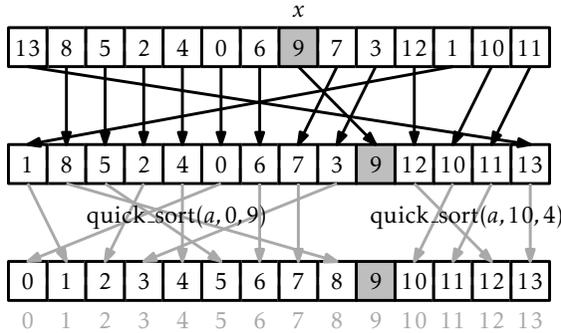
Figure 11.3: An example execution of `quick_sort(a, 0, 14)`
