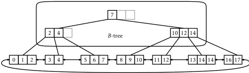
Figure 14.11: A  $B^+$ -tree is a  $B$ -tree on top of a doubly-linked list of blocks.
