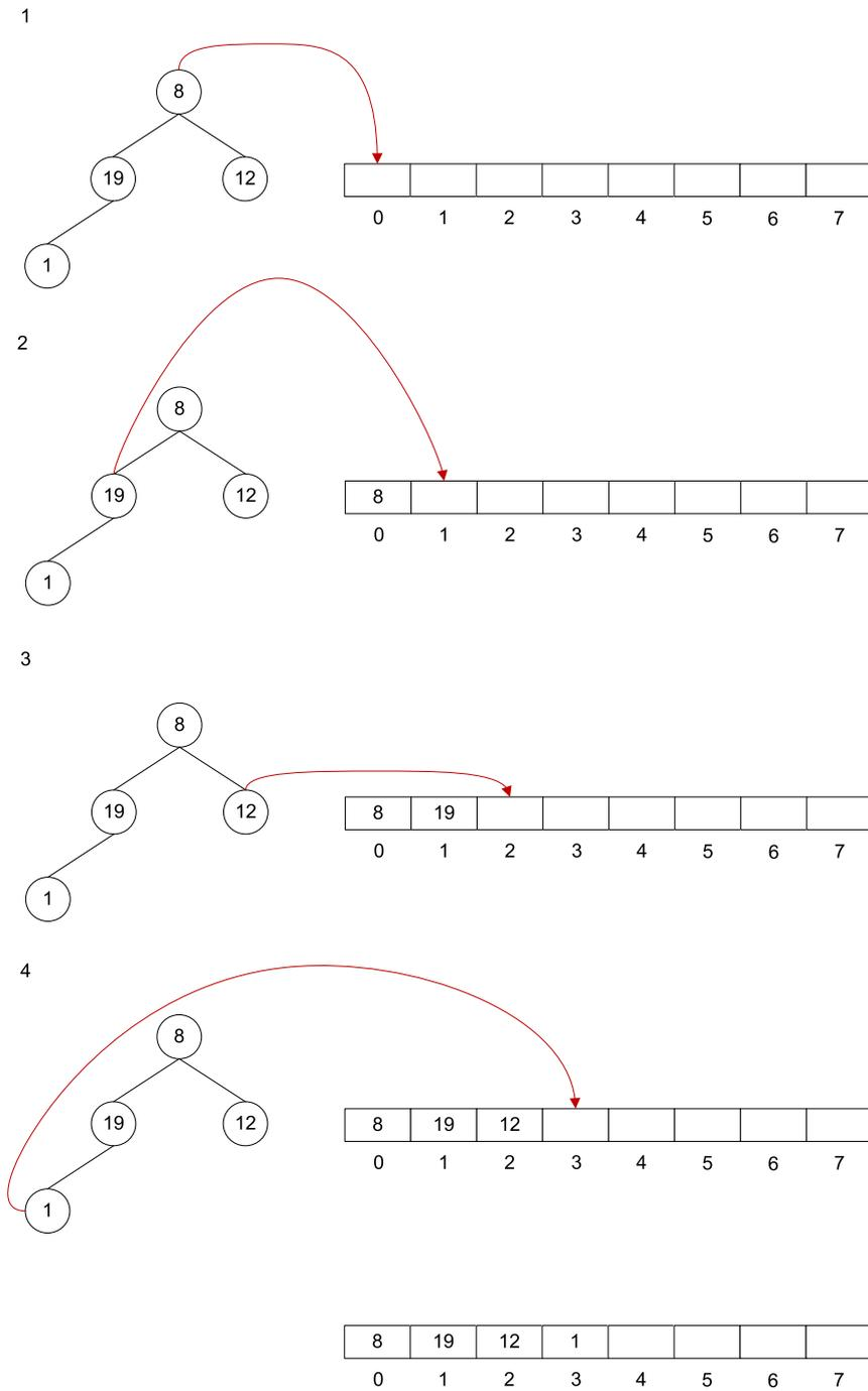
Figure 4.3: Converting a tree data structure to its array counterpart
