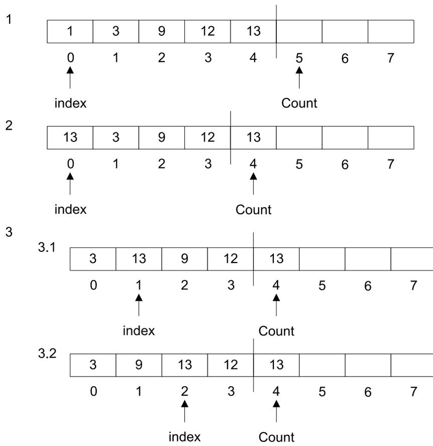
Figure 4.6: Deleting an item from a heap
