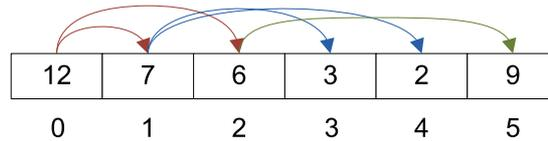
Figure 4.2: Direct children of the nodes in an array representation of a tree data structure
