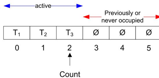
Figure 4.8: Living and dead space in the heap backing array
