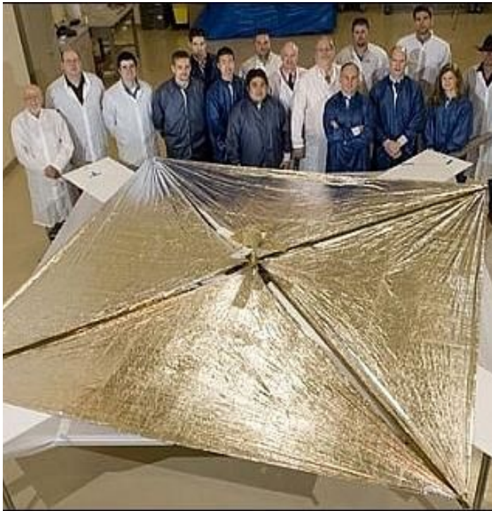
Figure 3: NanoSail-D2 ground deployment test (Source: NASA/MSFC)
