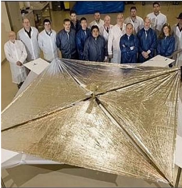
Figure 3: NanoSail-D2 ground deployment test (Source: NASA/MSFC)
