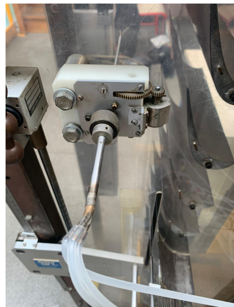
Figure 6: 3-inlet Pitot tube
