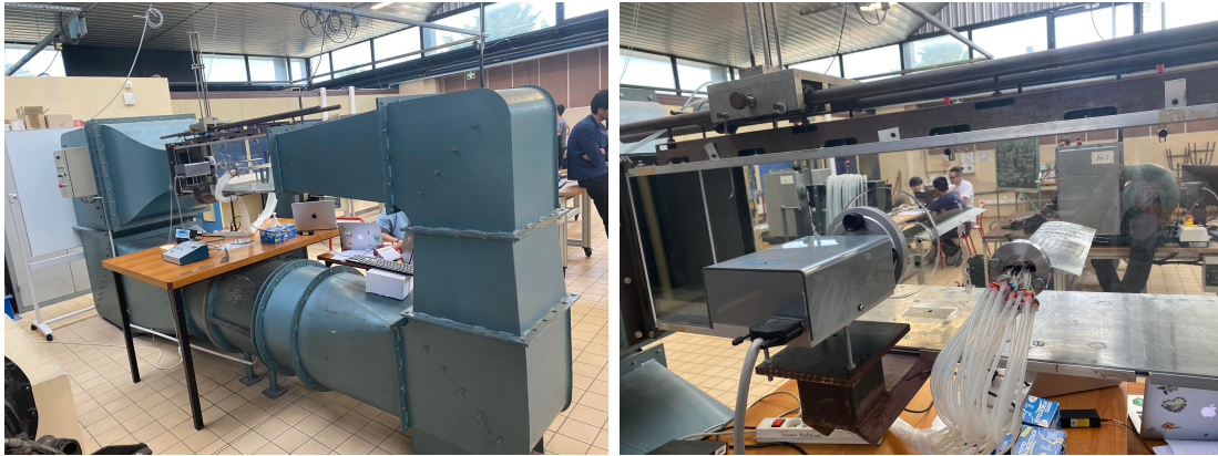
FIGURE 3 – Wind tunnel profile : complete experimental installation ( left ) and strain gauge balance ( right )
