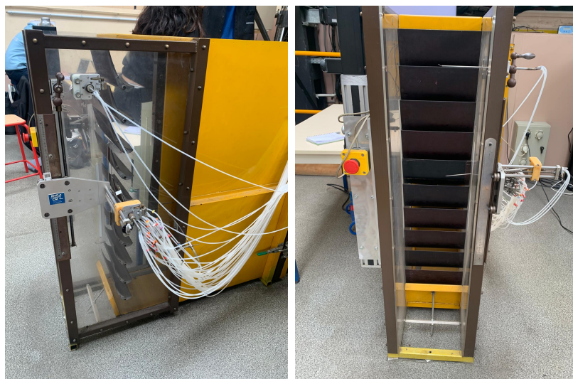
FIGURE 4 – Study of a blade grid : experimental installation
