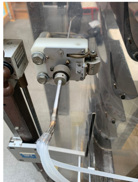
FIGURE 6 – 3-inlet Pitot tube
